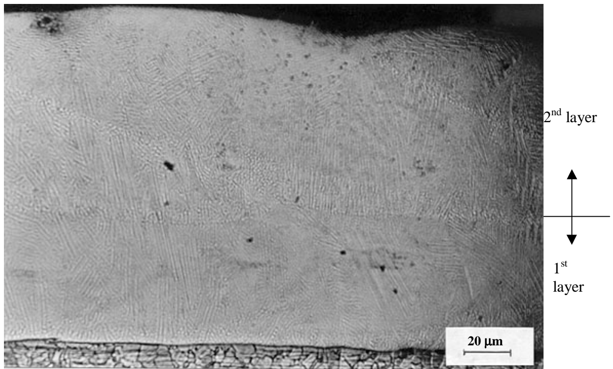
Figure 3 – Transverse cross section of the two layers laser cladded specimen, as observed under optical microscope.
